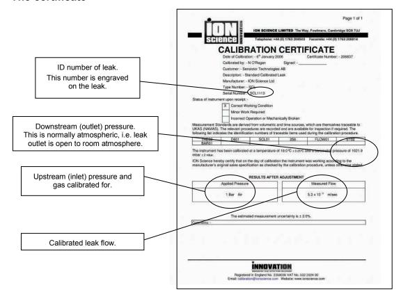
The first thing you must look at when setting up your leak is the leak specification. This must be correctly correlated to the data on the calibration certificate.
