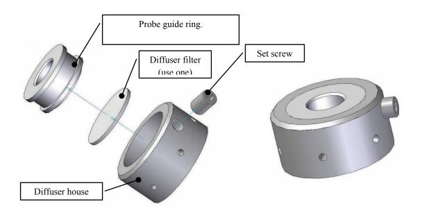
Install the leak in a panel if desired, or assemble diffuser and leak with red gasket as spacer. See figure below:
