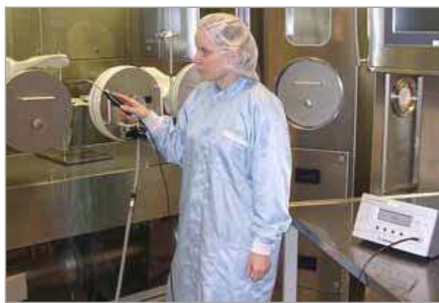
Fig. 1: Leak detection with Sensistor ISH2000 Hydrogen Leak Detector
